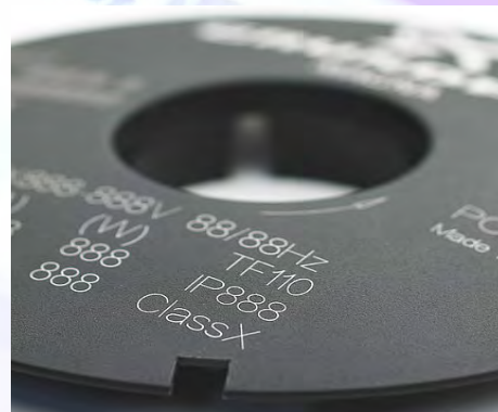
Laser engraving on ABS part
