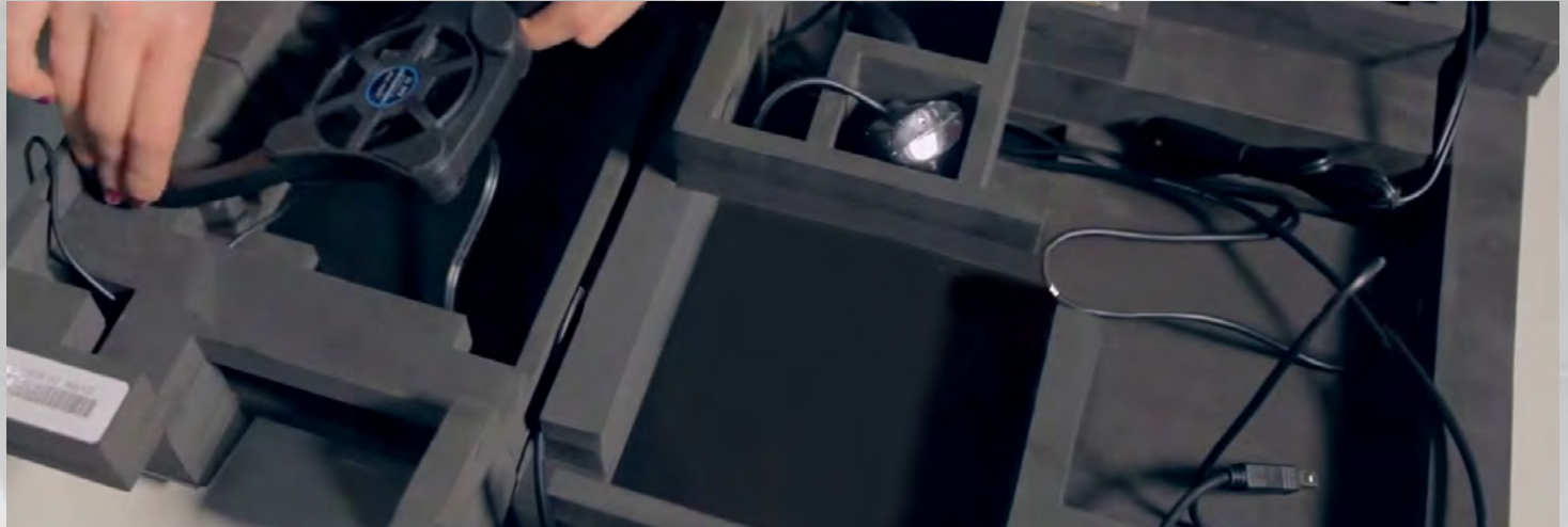
Assembly with pre-installed cable trunks for DC power and USB lines.
