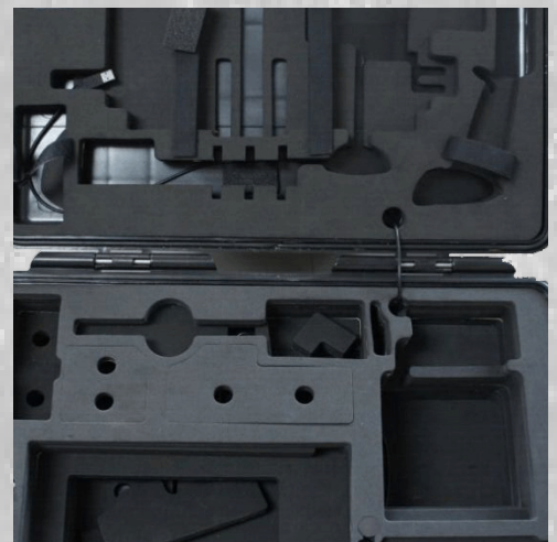
Complex EVA foam in lid & bottom / cable tree pre-installation
